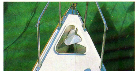
The large self draining anchor locker easily stows anchor and chain.
