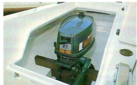
The outboard engine in its outboard well - "the inboard outboard".
