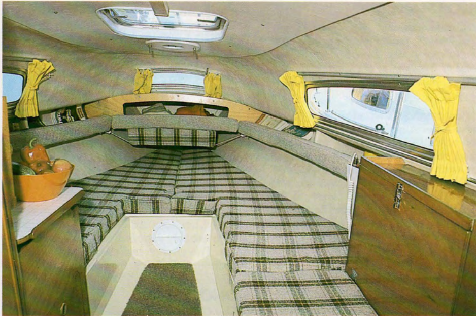
Looking for'ard with fold down sink, stowed away, galley top covering cooker. Toilet compartment port side, centre infill cushion stowed under for'ard shelf.
